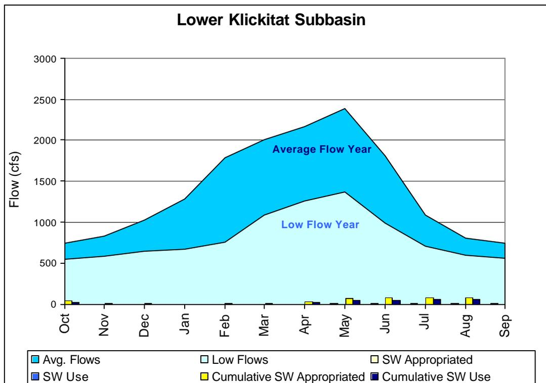
**Figure 9. Exceedance flows, water allocation and water use within the lower Klickitat subbasin (values of use and allocation within the subbasin are too small to show on the plot), and total cumulative water allocation and use reflecting water use in the Lower Klickitat subbasin and all upstream subbasins.**
