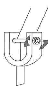
5. With the use of a \frac{1}{8} " socket or open end wrench, rotate in a clockwise manner wrapping the strap around the tension bolt
