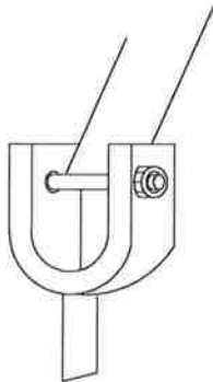
6. Once tensioned to the point that counter-clockwise resistance appears, a \frac{5}{16} " open end wrench should be used to hold the adequate neck while repositioning the \frac{1}{8} " wrench which will enable continued and final tensioning. Repeat as required
